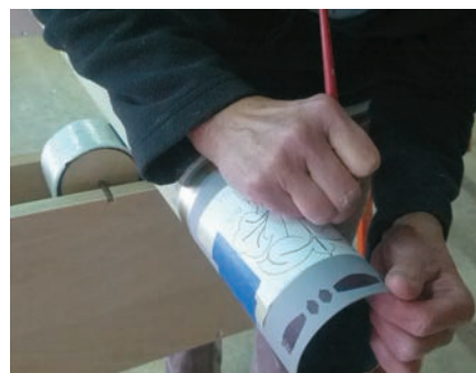
Pattern being transferred to the pipe
